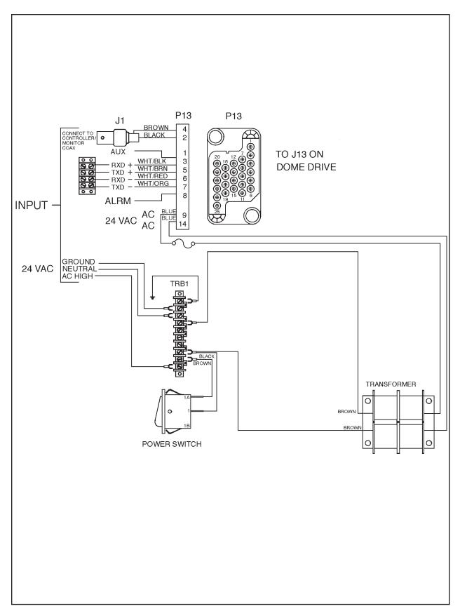
Figure 2. 24 VAC Back Box Wiring Diagram
